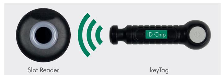
Being “Contact-Free” the radio wave can penetrate most non-metallic materials and by its very nature unlike contact based systems means there is no wear and tear of electrical parts. Again a typical common use that is fast disappearing is the old swipe card used for access control and credit cards where the daily constant swiping action through the reader caused endless problems with wear and tear. Dirt and damage on the card all took its toll, with RFID all this is eliminated. ▶
