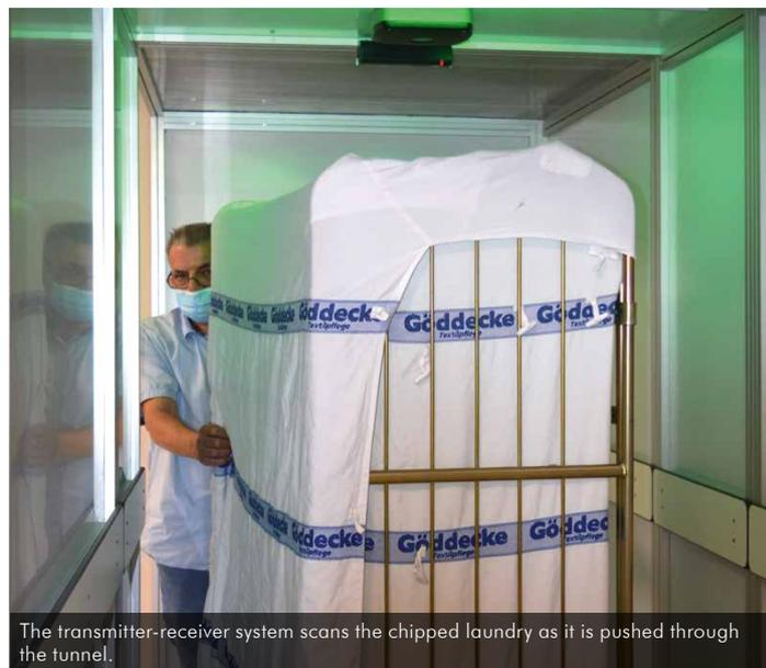
The transmitter-receiver system scans the chipped laundry as it is pushed through the tunnel.
