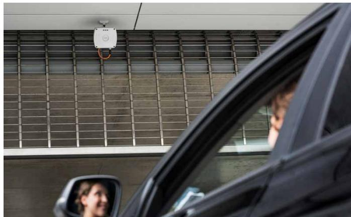
Another product from deister, the tranSpeed, allows fast, reliable and automatic wide-range identification of drivers and vehicles in the entrance and exit areas. This system is also controlled via the Commander Connect software. Car drivers benefit from automatically opening gates – a plus point in terms of comfort and security.
