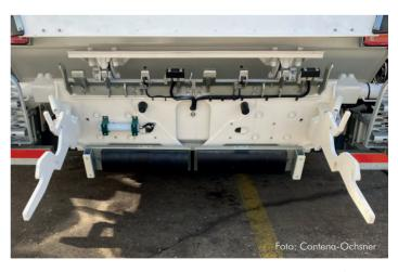
as time and cost savings through the accurate identification of the number of bins and waste weight. Precise identification of waste weight ensures accurate calculation of waste collection costs. The bins are fitted with a transponder that are read directly at collection via a comb or body antenna mounted on the vehicle. The body antennas implemented in this project ensure all waste containers equipped with HDX and FDX transponders can be quickly and reliably identified,
